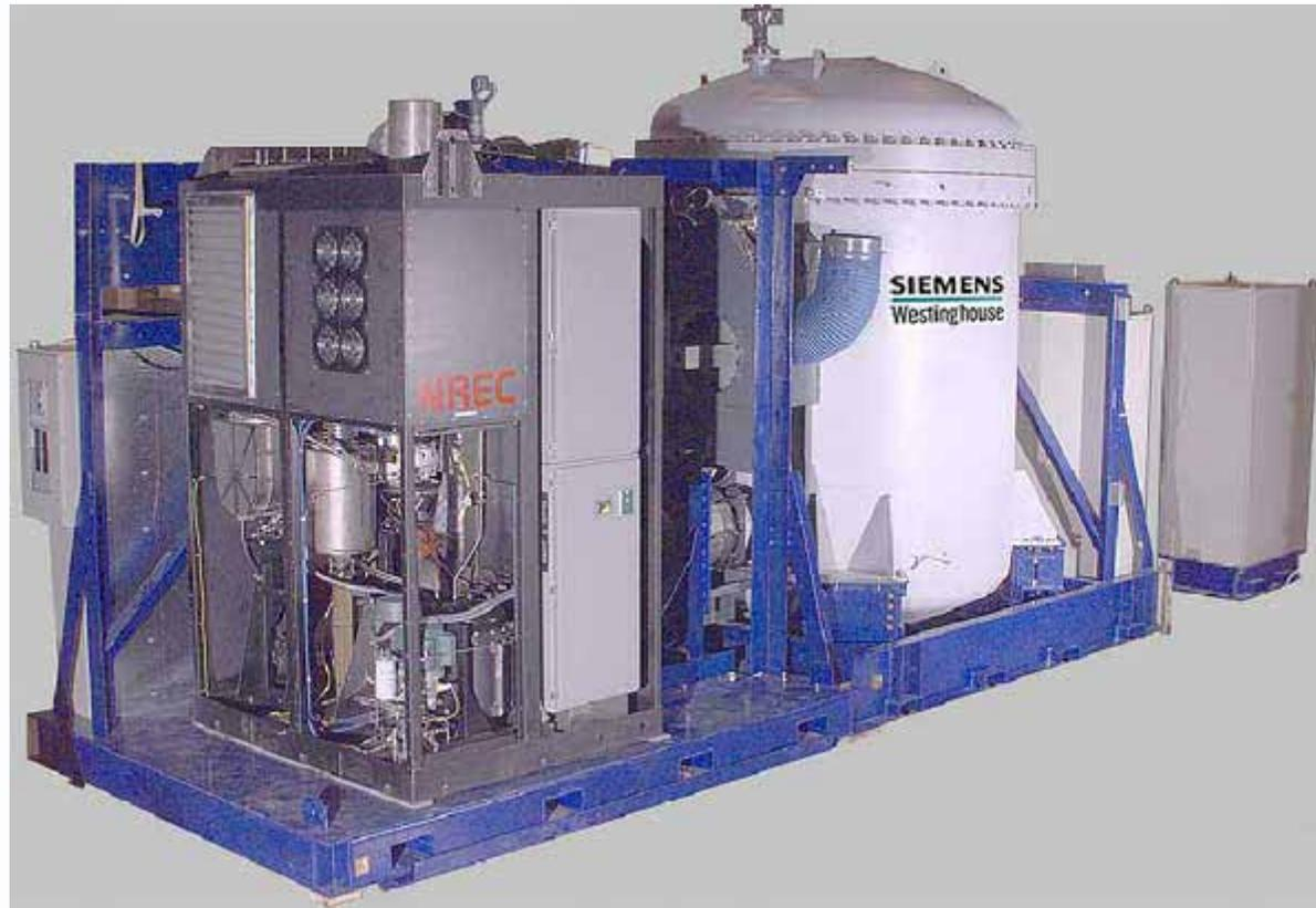
**Siemens Westinghouse SOFC/Gas Turbine Hybrid 220 kW**
