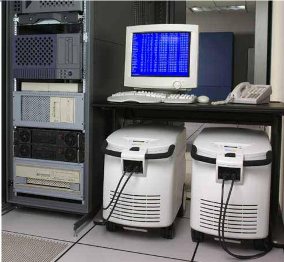
Based around Ballard's 1.2kW PEM fuel cell power module, these systems are designed for industrial use as a portable power generator or emergency back up power system. Its retail price is US\$5,995. It is fuelled by compressed hydrogen, although another option - hydrogen stored in metal hydride canisters - has been extensively explored and should be offered soon.
